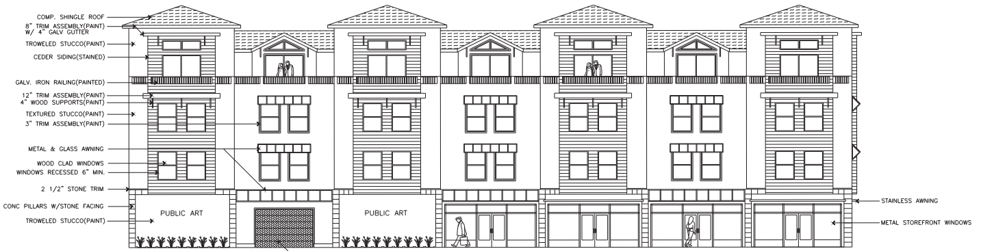
SOUTH ELEVATION NOTE: ALL FINISHES ARE THE SAME AT ALL ELEVATIONS UNLESS OTHERWISE INDICATED.
